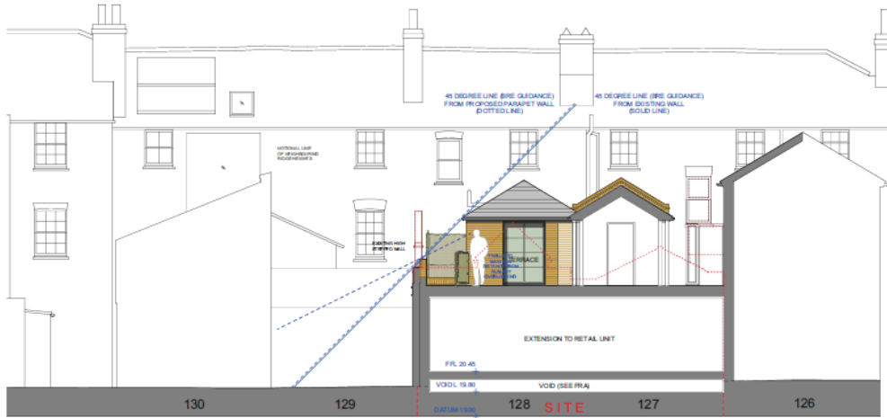
SIDE TERRACE ELEVATION / SECTION E-E
